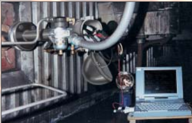
Infra-View ® Boiler Thermometer maintenance and customization being performed with a laptop computer in the field. Sensor programming can be accomplished anywhere along (2) wire loop or at DCS.
