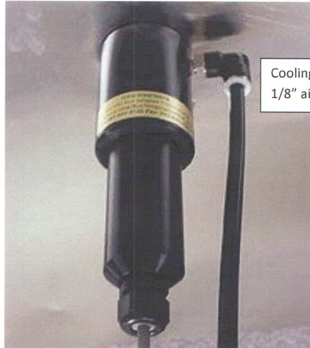
2 wire signal line for 4 – 20 mA output
